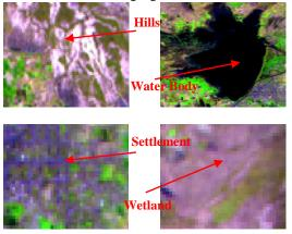
Fig. 4. Image Pixel Identification for Signature File Creation
